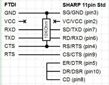
PC-E220 and PC-G850 setup: Menu TEXT->Sio->Format baud rate = 9600 data bit = 8 stop bit = 1 flow = RS/CS
